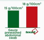
Evaluates the total absorptive capacity after 30 minutes of immersion at 37°C (without any compression).
