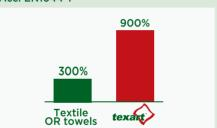
Evaluates the water absorption capacity by difference of mass before and after water immersion and draining without compression.
